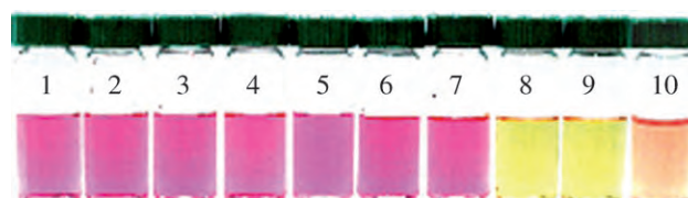
Figure 2. Color changes of the ethanol/water solution of L - \text{Hg}^{2+} in the presence of different amino acids. Labeled vials: 1) no amino acid, 2) Gly, 3) Leu, 4) His, 5) Glu, 6) Asp, 7) Met, 8) Cys, 9) Hcy, and 10) GSH. [\text{L}] = 1.0 \times 10^{-4} \text{ M} , [\text{Hg}^{2+}] = 2.5 \times 10^{-4} \text{ M} , [\text{amino acid}] = 1.0 \times 10^{-3} \text{ M} .
